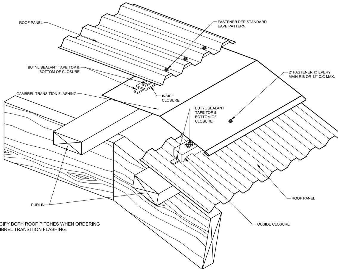
NOTE: SPECIFY BOTH ROOF PITCHES WHEN ORDERING GAMBREL TRANSITION FLASHING.
