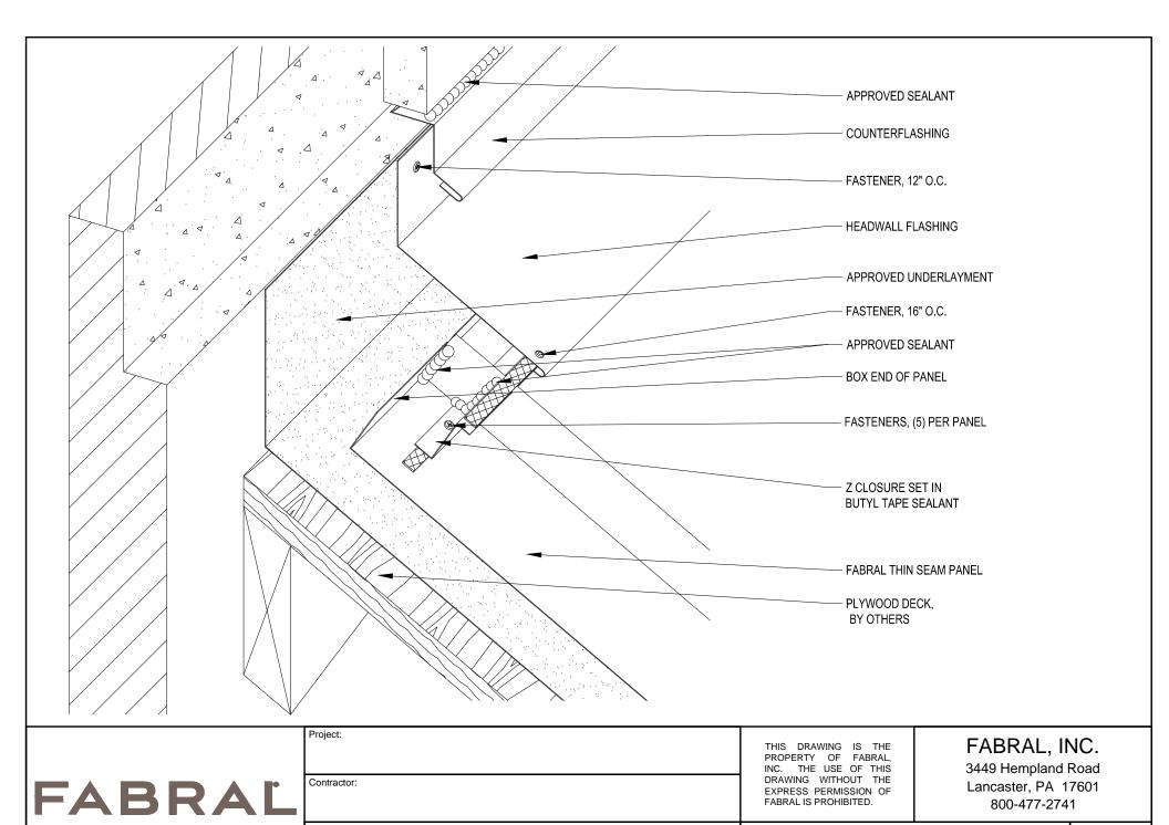
**HEADWALL (ENDWALL) DETAIL (HW-2)**
