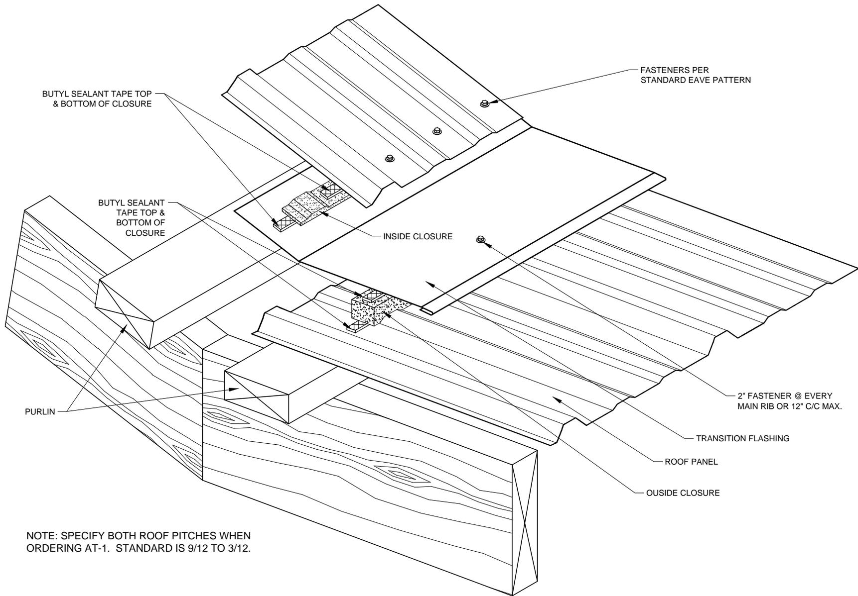
NOTE: SPECIFY BOTH ROOF PITCHES WHEN ORDERING AT-1. STANDARD IS 9/12 TO 3/12.
