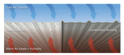
CONDENSTOP SHOULD ONLY BE USED ON OPEN FRAMING JOBS.
