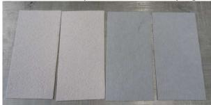
Picture of the samples after the 1,000 h. temperature exposure (beige + grey)
