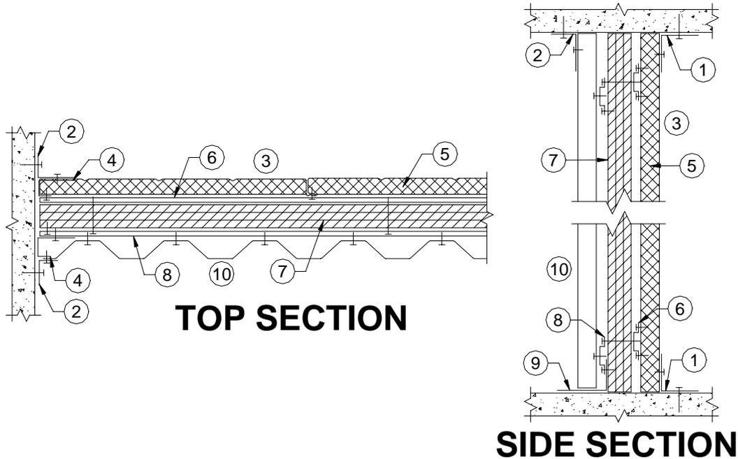
1. Steel Supports: 3" x 3" x 1/4" steel angles attached to masonry with 3/8" x 2" steel bolts with expansion shields.
