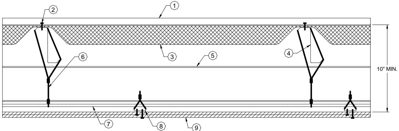
1. Metal Roof Deck Panels: 26 ga. minimum steel. Panels continuous over two or more spans. End laps to occur over purlins with panels overlapped a minimum of 4". Sealant may be used at panel side and end laps. Panels must have UL 90 uplift rating with steel purlins.
