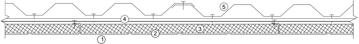
1. 22 ga. steel LP-15, perforated  $\frac{1}{8}$ " diameter holes on  $\frac{3}{8}$ " centers.
