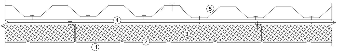
1. 22 ga. steel LP-25, perforated  $\frac{1}{8}$ " diameter holes on  $\frac{3}{8}$ " centers.
